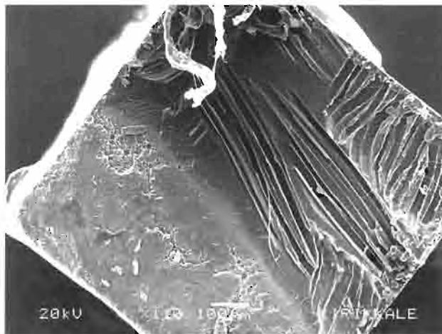
Fig 5 Composite side of a debonded specimen in the high c-factor group in which mixed failure occurred. Specimen was restored with everStick NET. The structure of the fiber material was destroyed during the specimen preparation.
